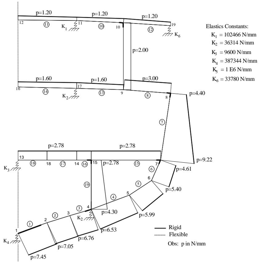
Fig.2 - Transverse structure
